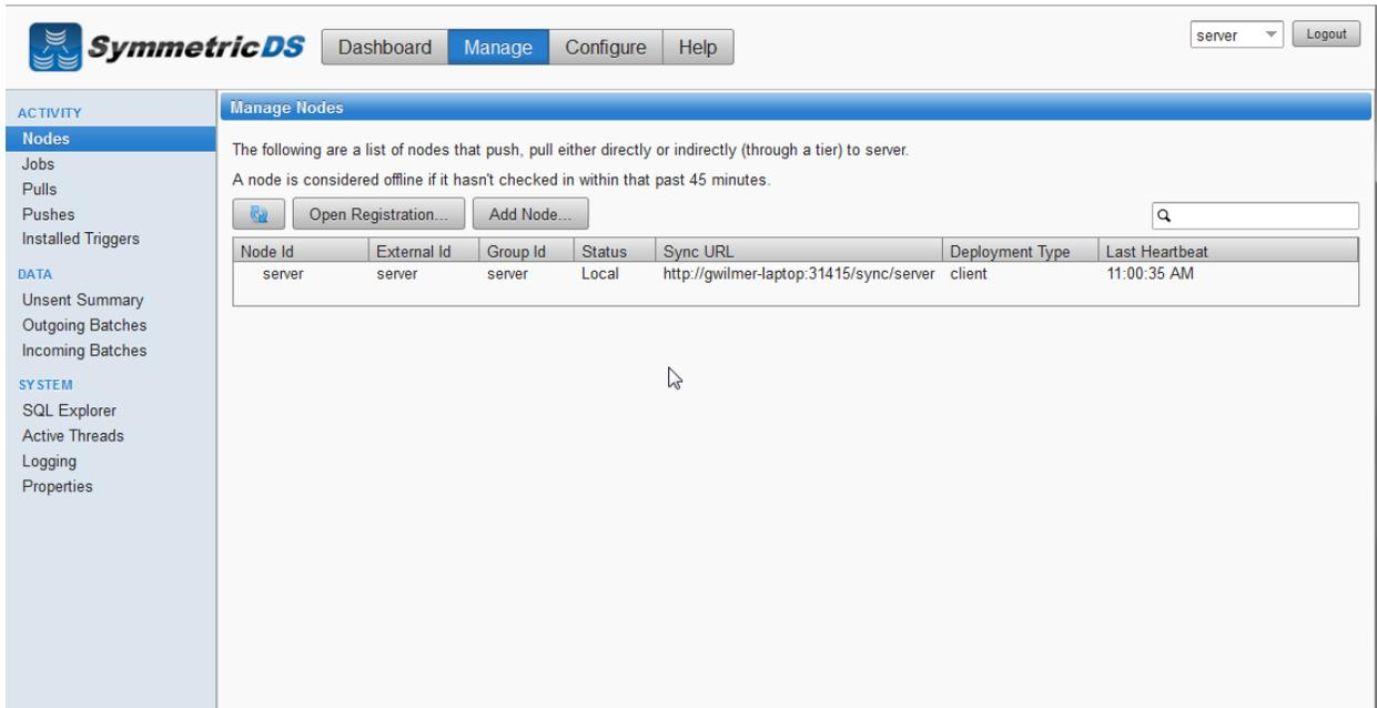
The screenshot shows the SymmetricDS web interface. The top navigation bar includes 'Dashboard', 'Manage', 'Configure', and 'Help'. The 'Manage' menu is active. On the left, there is a sidebar with 'ACTIVITY' and 'SYSTEM' sections. The main content area is titled 'Manage Nodes' and contains the following text:
