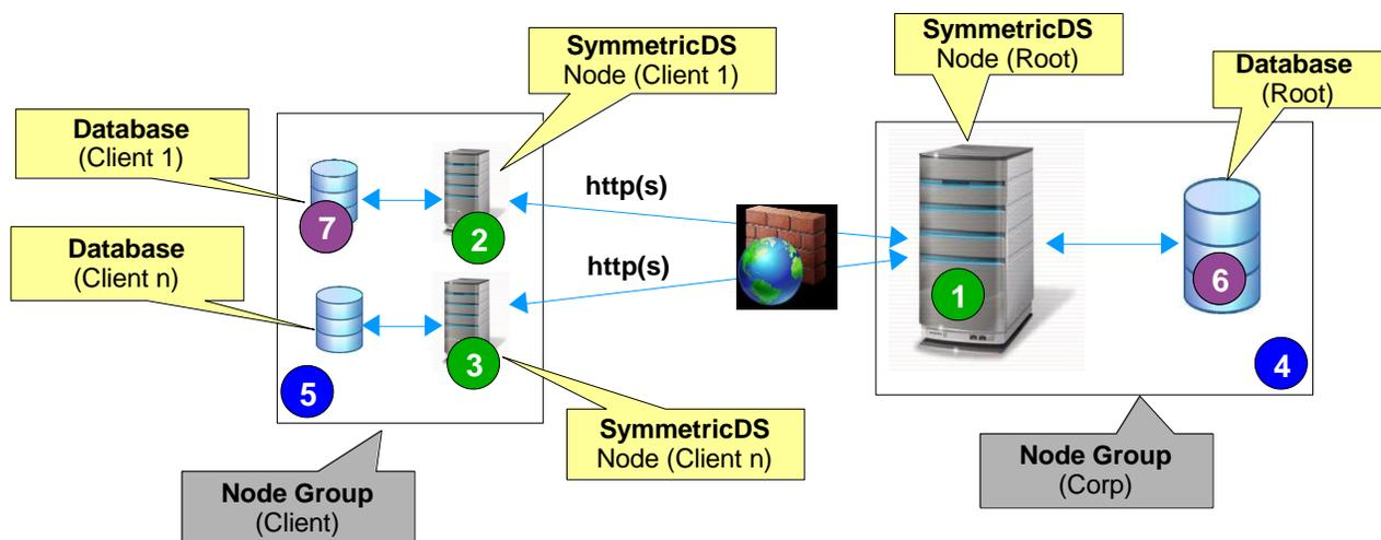
In the retail scenario on the previous page, each database has its own instance of symmetric running on a server that is attached to the database (#1, #2 and #3). This one to one relationship between symmetric instance and database is called a single-homed setup.
