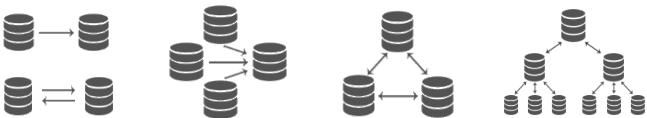
Figure 4: Multiple use cases are possible, including 1-way, bi-directional, one source to multiple targets, multiple sources to one target, multi-master, and tiered replication.
